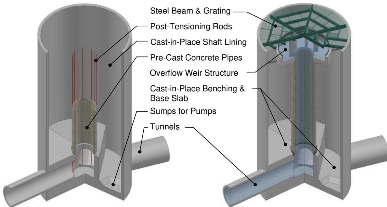
Figure 5. Construction Sequence of the Overflow Structure.
