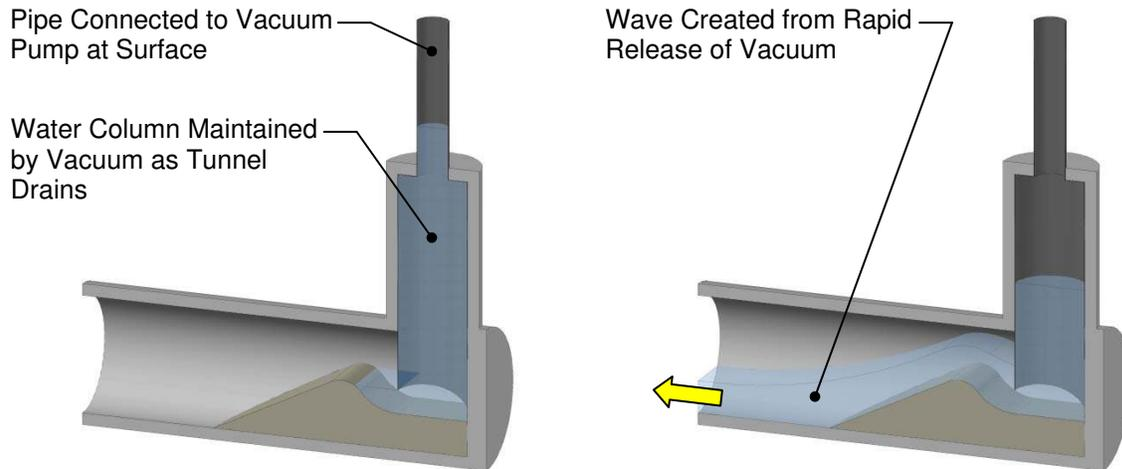
Figure 4. Flushing System.
