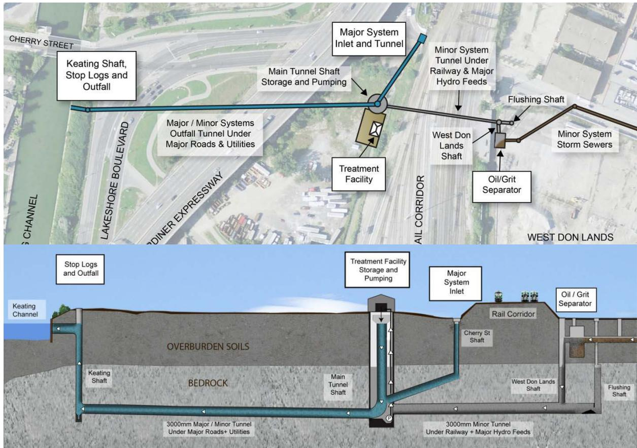
Figure 1. Storm Water Conveyance System.
