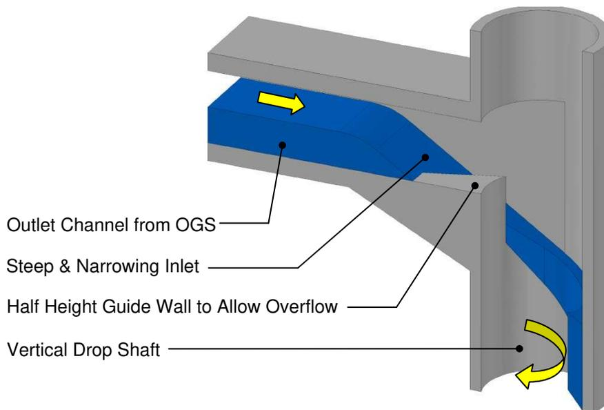
Figure 3. Vortex Drop Shaft.
